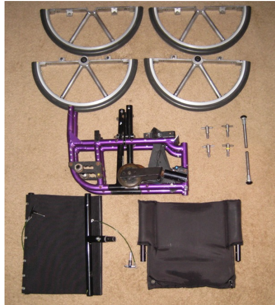
Photo 2: This picture shows the components of the wheelchair when disassembled. The 20" circular wheel is disassembled into two semi-circular parts.
